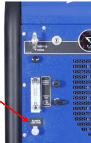
Figure 4-4. Location of Blower Lube Port
