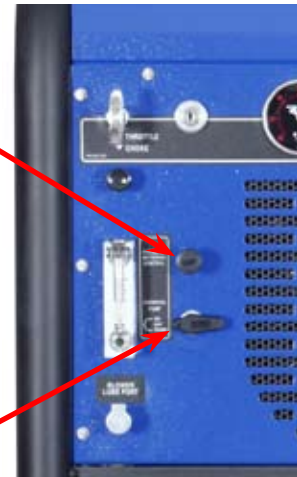
Figure 4-3. Location of Chemical Metering Control and Chemical Pump Selector Valve
