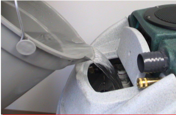
Pour appropriate amount of hot water into solution tank
