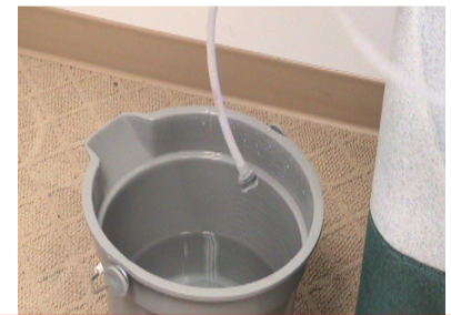
Place Chemical Feed Hose into Rinse Solution
