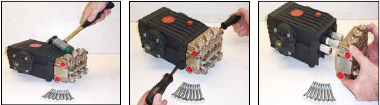
Figure 5-6. Separate Manifold from Crankcase
