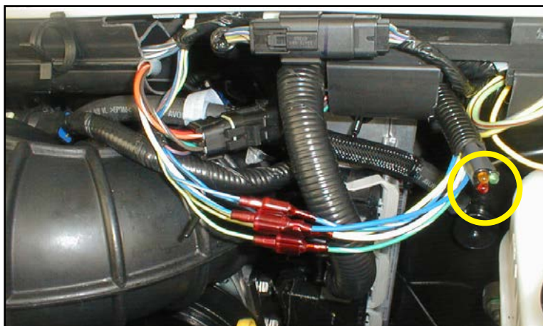
Figure 3-2. Location of 3 Lights on Throttle Control Assembly
