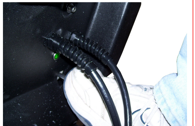
PRESSING THE PUMP PRIMING VALVE
