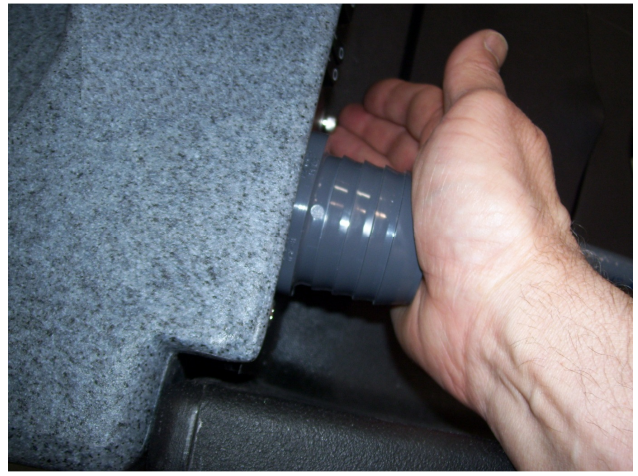
BLOCKING THE VACUUM PORT TO PRIME THE PUMP
