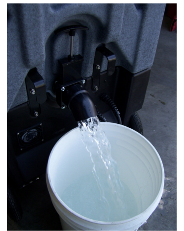
Draining the Recovery Tank
