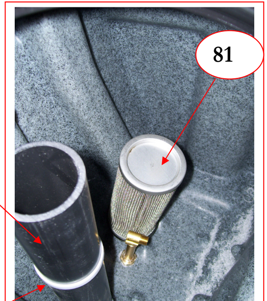
INSIDE RECOVERY TANK WITH PUMP-OUT FILTER IN PLACE
