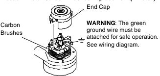
Note: When replacing carbon brushes loosen wire terminal BEFORE removing screws on bracket.
