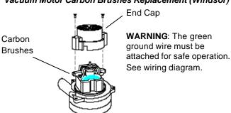
If armature commutator is grooved, extremely pitted or not concentric, the motor will need to be replaced or sent to a qualified service center.
