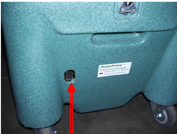
PUMP PRIMING VALVE
