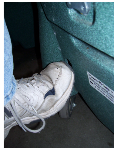
PRESSING THE PUMP PRIMING VALVE
